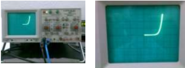
Figure 11, 10x10 Cm 2 Solar Cell I-V Test Results, X-axis: 0.2V/div, Y-axis 1A/div
