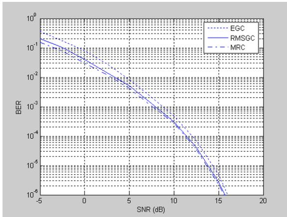
Fig. 2 BER for RMSGC, MRC, and EGC combining techniques using 8 antennas
