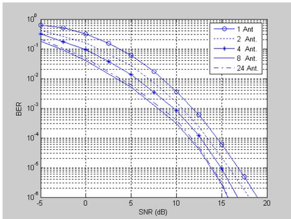
Fig. 3 BER for RMSGC using different antenna numbers
