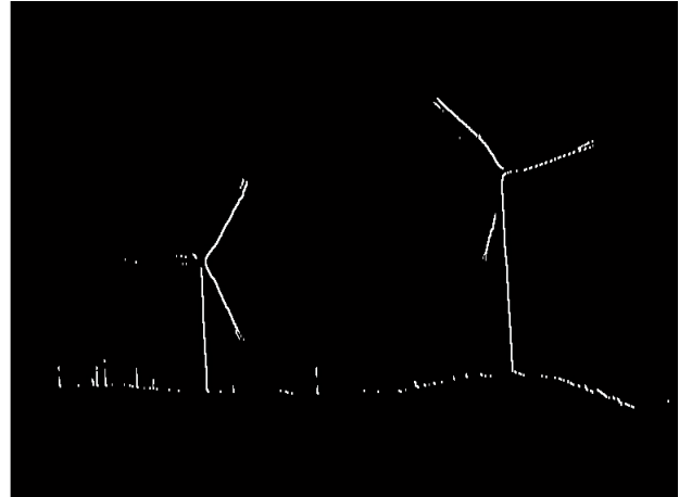
Figure 3: By applying the Prewitt Filter, the most of the background is removed, keeping vertical regions of the image.
