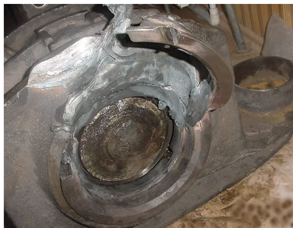
Figure 5. The fracture of bearing box as a result of heat disipated from friction against the locking ring.
