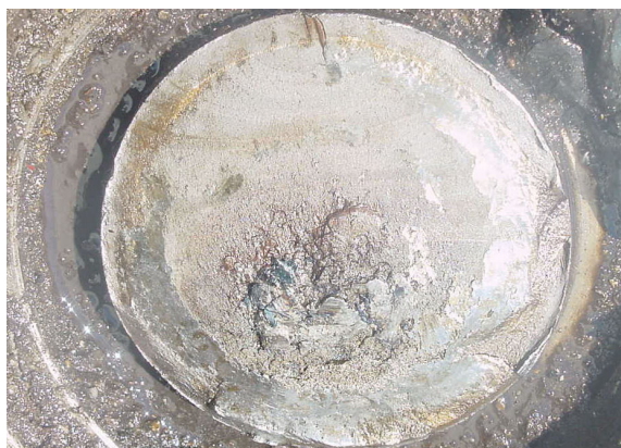
Figure 1. Broken tank wagon axle from a severe derailment.
