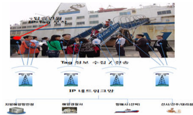
Fig. 5 Concept Diagram of IP-RFID-based Person Management
