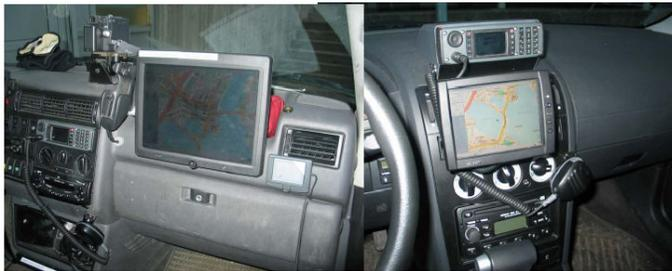
Fig. 2 Vehicle installations of the POKE system [6]
