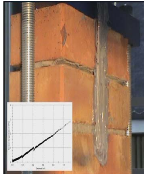
Fig. 4 Bonding test GFRP strip-masonry block
