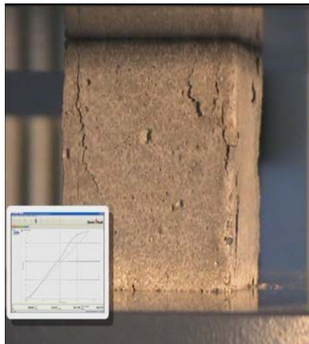
Fig. 2 Compression test on mortar specimen
