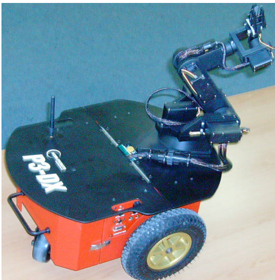
Fig. 6. Mobile platform Pioneer 3-DX WMR.
