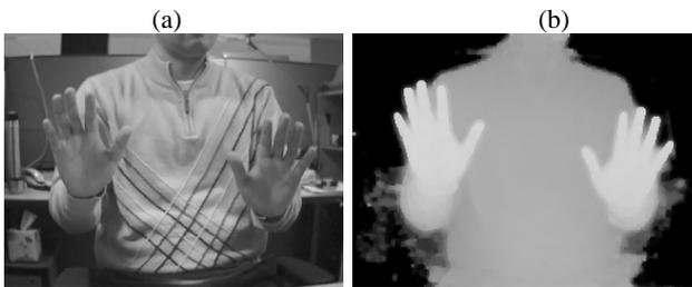
Fig. 3 (a) input image; (b) disparity image
