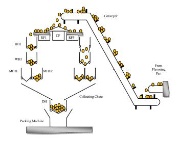
Fig.1 Production Chain: Conveyor - Combinatorial Weigher - Packing Machine
