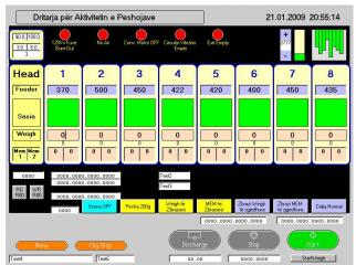
Fig. 6 Operating screen with weight state of each head
