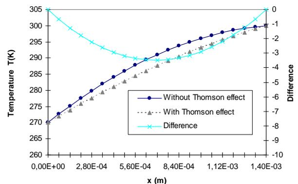
Figure 4 : Comparison of the temperature field obtained with or without the Thomson effect
