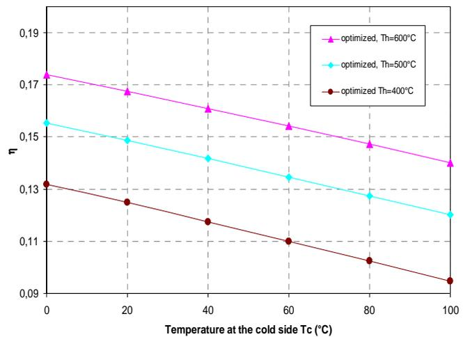
Figure 11: Influence of the cold side temperature on the efficiency of the p-leg for three different temperatures at the hot side
