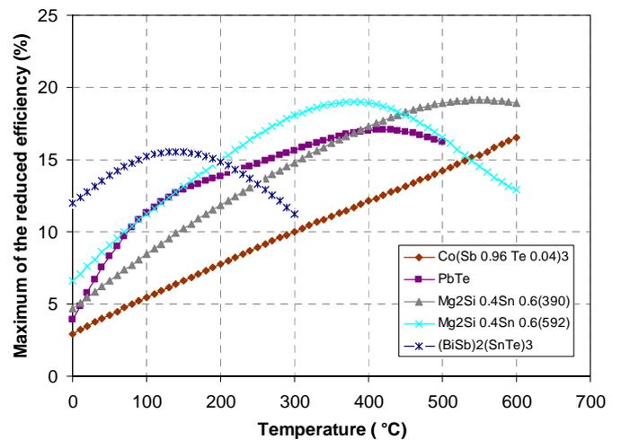
Figure 8: Maximum of the reduced efficiency for n-type materials
