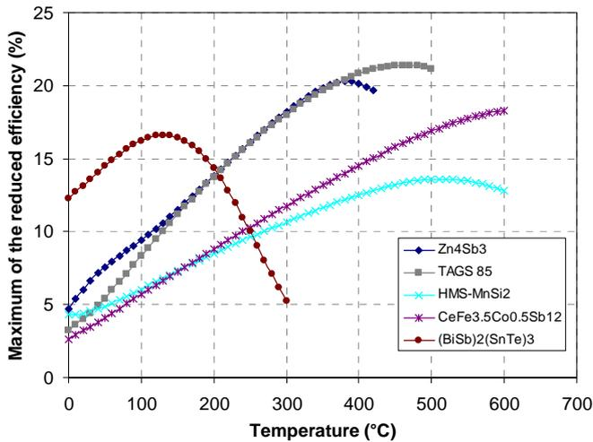
Figure 9: Maximum of the reduced efficiency for p-type materials
