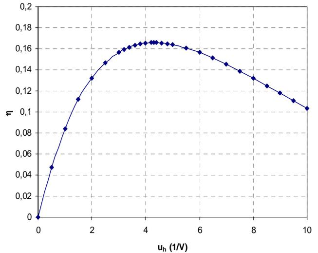
Figure 10: Efficiency as a function of the relative current density value at the hot side
