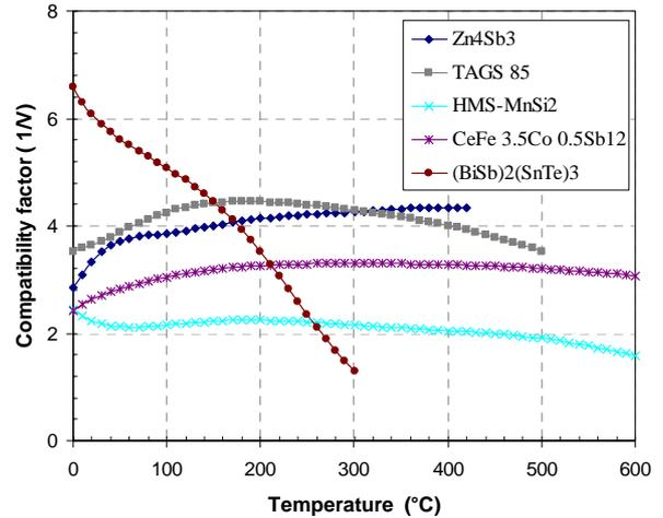
Figure 7: Compatibility factors for p-type materials
