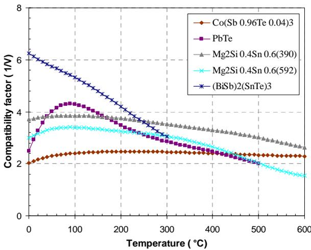
Figure 6: Compatibility factors for n-type materials
