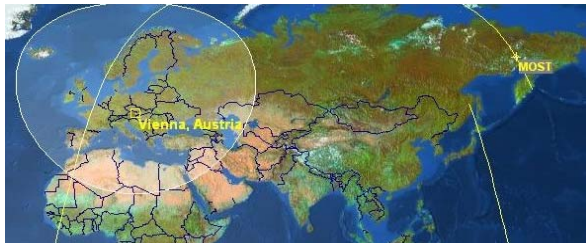
Fig. 9. Visibility region of Vienna ground station for elevation angle of 0^\circ [11].
