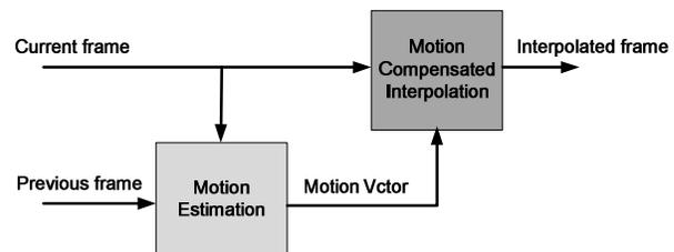
Fig. 1. Block diagram of MC-FRUC.
