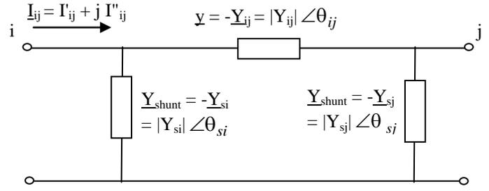
Fig. 1 – Transmission Line Model
