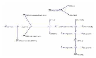
*Figure 4*: Electrical operation of a lathe by using PI type regulators with solved causality in Bondin ©.
