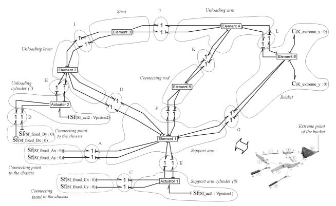
Figure 7: Front-loader mechanism by using subsets in Bondin ©.
