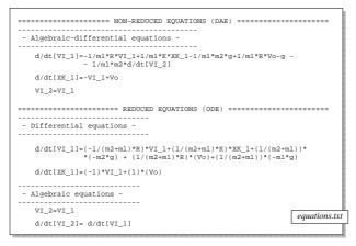
*Figure 5*: File with equations obtained from a model composed by two inertances with a rigid union.
