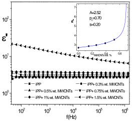
**Figure 7**: Real part of the dielectric function ( $\varepsilon'$ ) vs frequency for series iPP / MWCNTs. The inset shows static permittivity  $\varepsilon'$  vs MWCNTs concentration *p* for nanocomposites below  $p_c$ . The line is a fit of eq. (3) to the experimental points.
