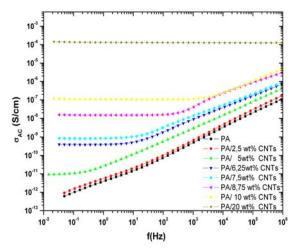
**Figure 4 :** Conductivity vs frequency for PA6/MWCNTs samples
