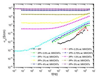
**Figure 6**: Conductivity vs frequency for series iPP / MWCNTs and for the samples indicated on the plot.
