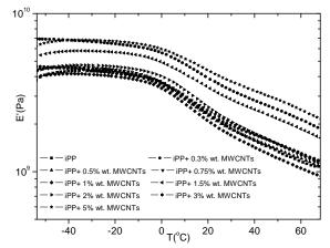
**Figure 2**: Storage modulus E' vs temperature for series iPP / MWCNTs
