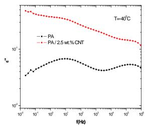
Figure 9 : Imaginary part of the dielectric function ( $\epsilon''$ ) versus frequency at -40 °C for PA6/MWCNTs
