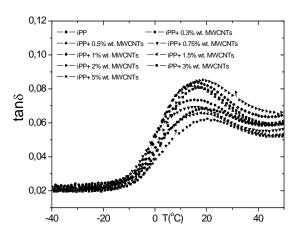
Figure 3: Loss tangent vs temperature for series iPP / MWCNTs
