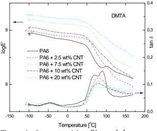
Figure 1: Storage modulus E' and loss tangent (=E''/E') vs temperature for series PA6 / MWCNTs
