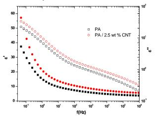
**Figure 10 :** Real part ( $\varepsilon'$ ) (filled symbols) and imaginary part ( $\varepsilon''$ ) (open symbols) of the dielectric function versus frequency at room temperature for the samples indicated on the plot.
