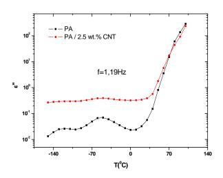
**Figure 8 :** Imaginary part of the dielectric function  $(\varepsilon'')$  versus temperature at a frequency of 1.19 Hz for the samples indicated on the plot.
