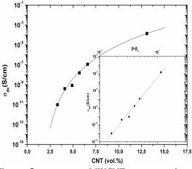
**Figure 5 :**  $\sigma_{dc}$  vs MWCNTs concentration p for PA6/MWCNTs nanocomposites above  $p_c$ . The inset shows a log-log plot of  $\sigma_{dc}$  vs (p-p<sub>c</sub>) with t = 8.4 and  $p_c=1.7$  vol. %.
