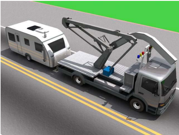
Figure 1: Visual representation of the system. The sensors are mounted on an articulated arm placed on a truck. All command and control is made at distance using a dedicated equipment mounted inside a Mobile Control Center (MCC)
