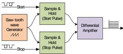
**Fig 1. Block Diagram of Saw-tooth Wave Based TDC**
