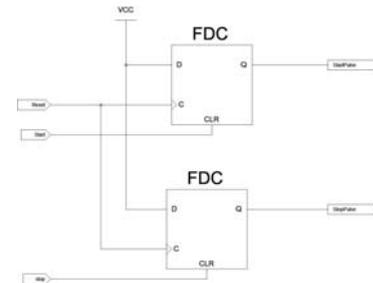
**Fig 4. Flip-flop Circuit for Synchronizing Signals**
