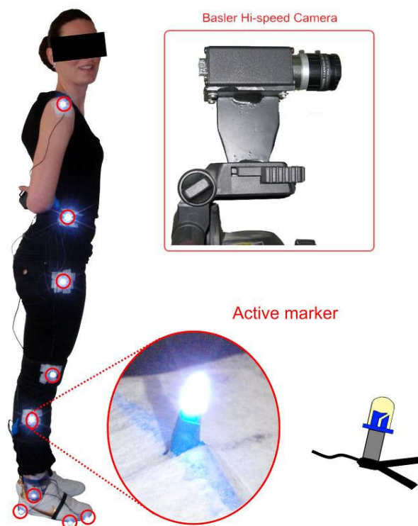
Fig.1, Subject with attached active markers (left), fast industrial camera Basler 602fc (top) and magnified active marker (bottom)
