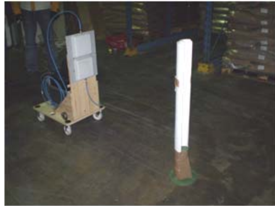
Fig.3. The test set-up for Gen2 tag measurements in cold circumstances
