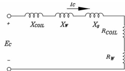
Fig.1 Load model for induction heating
