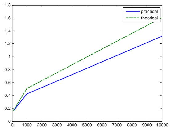
Fig.2 Theoretical and experimental diagram of load resistance variations (Ohm) vs. frequency variations (Hz)
