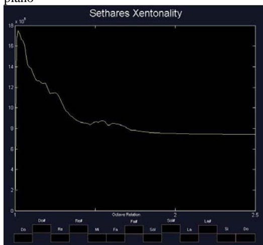
Fig. 9 Dissonance Curve for a Resonance of piano
