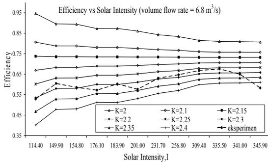
Fig. 3(a): Relationship between collector's efficiency and solar intensity with different  $K$  values (volume flow rate =  $6.8 m^3/s$ )
