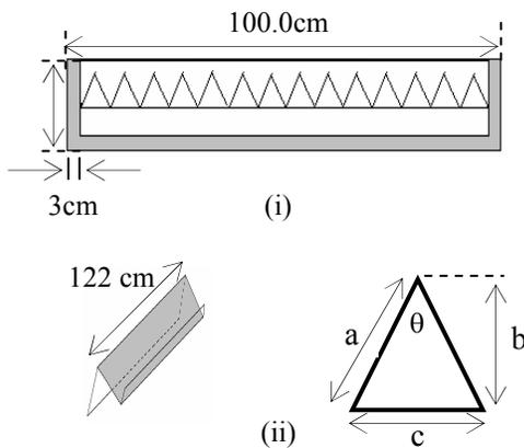
Fig. 1: (i) Cross-section of the V-groove solar collector; (ii) V-groove absorber design
