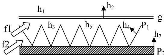
Fig. 2: Schematic of V-groove flat plate solar air collector showing energy balance
