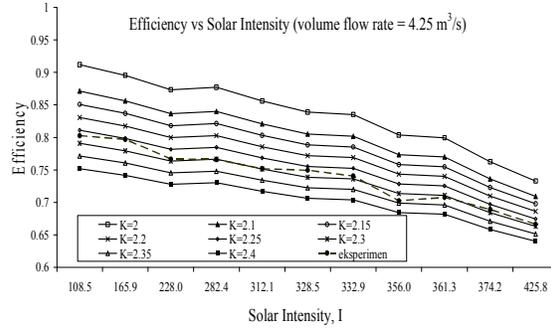
Fig. 3(b): Relationship between collector's efficiency and solar intensity with different  $K$  values (volume flow rate =  $4.25 m^3/s$ )
