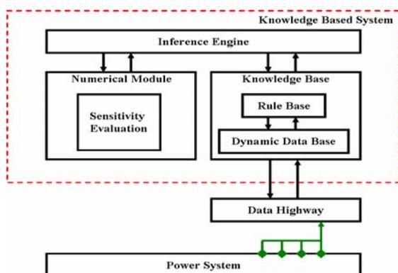
Fig. 1 Structure of intelligent voltage control system
