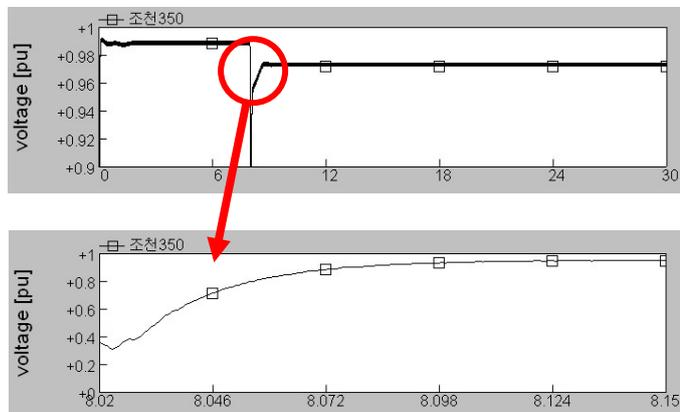
**Fig. 6** Voltages of Jocheon (350) bus by elapsed time after the voltage control has been applied
