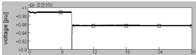
**Fig. 5** Voltages of Jocheon (350) bus by elapsed time before the voltage control has been applied
