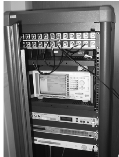
Fig. 3. DVB-T transmission system.
