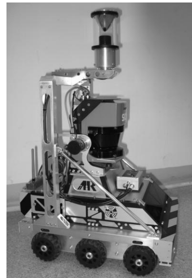
Fig. 2. Robot "Elektron" with 3D laser on a rotating head.
