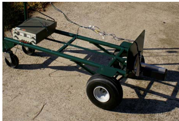
Fig. 16. Test cart to provide static height.
