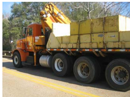
Fig. 1. Tri-axel test truck loaded with concrete filled weights.
