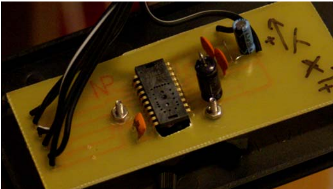
Fig. 7. Prototype I - ADNS-3060 with support circuitry.
