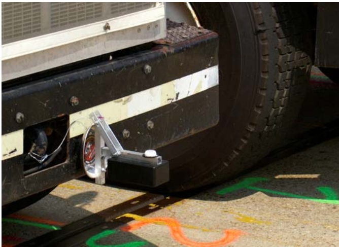
Fig. 6. Prototype I mounted magnetically to an ALDOT test vehicle.
