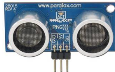
Fig. 9. Ultrasonic rangefinder used in Prototype II for automatic height sensing.
