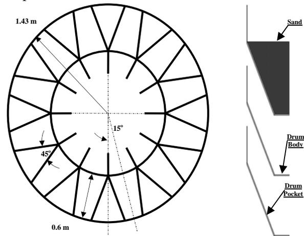
Figure 6: Cross sectional view in the cooling drum with the 2-D approximation
