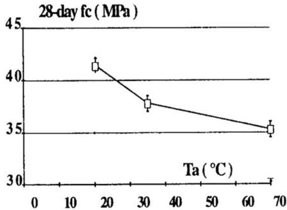
Figure 1: Effect of aggregate temperature on the 28-day concrete compressive strength [3].
