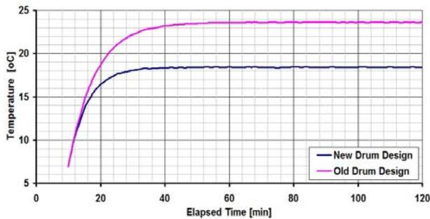
Figure 8: Average temperature of the sand at the drum exit.
