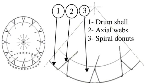
Figure 3: Detailed drawing of a cross section in the cooling drum
