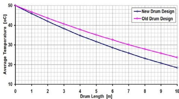
Figure 9: Sand temperatures through drum pockets.
