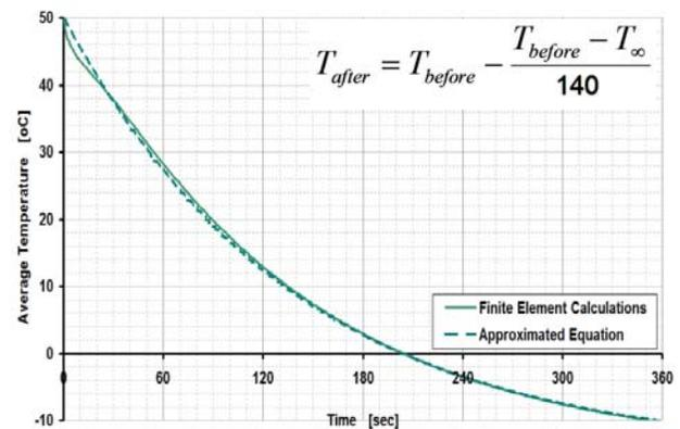
Figure 11: The Sand falling simulation model results and the empirical equation.
