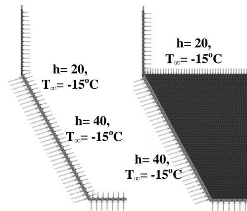
Figure 7: FE model and boundary conditions of the empty and filled pockets
