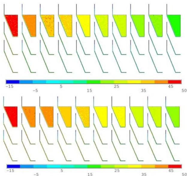
Figure 10: Sand temperature distribution through drum pockets.
