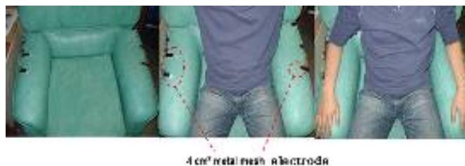
Fig. 6. A photography of ECG eletrode attached on a sofa.
