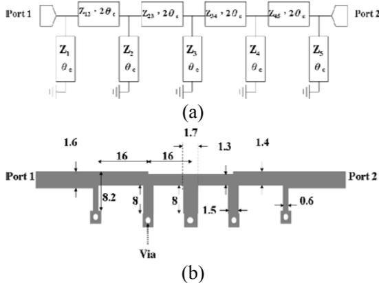
Fig. 1. (a) General circuit model for the proposed UWB BPF without coupled feed lines and (b) the layout of the UWB filter.
