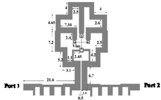
Fig. 7. Layout of the improved UWB BPF with embedded bandstop structure in input/output (I/O) lines to have a wide stopband.
