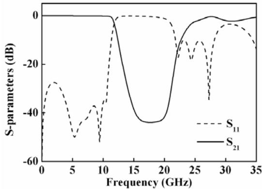
Fig. 6. Frequency response of the optimum bandstop filter shown in Fig. 5.
