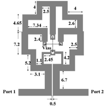
Fig. 3. Layout of the compact UWB BPF by bending the short-circuited stubs and coupling the I/O feed lines.
