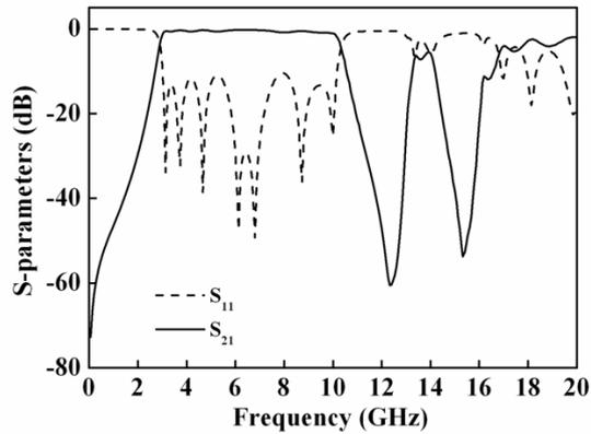
Fig. 2. Frequency response of the UWB filter as shown in Fig. 1(b).
