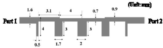
Fig. 5. Layout of the bandstop filter using five open-circuited stubs.
