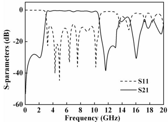
Fig. 4. Frequency response of the UWB filter with the bended structure.
