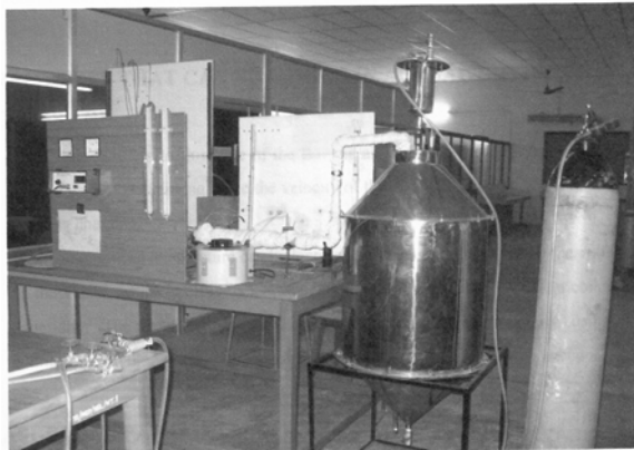
Fig. 1a: Overall setup of spray dryer
