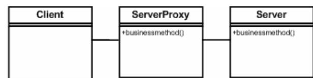
Fig. 3 Proxy Pattern Class Diagram
