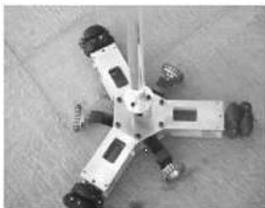
Fig. 2. Omni-directional chassis.
