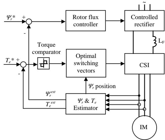
Fig. 1. DTC of CSI drive based on hysteresis control
