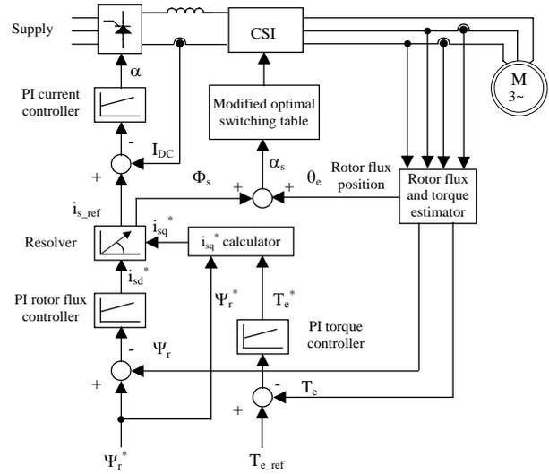
Fig. 4. Constant-switching DTC strategy in CSI fed induction motor drive
