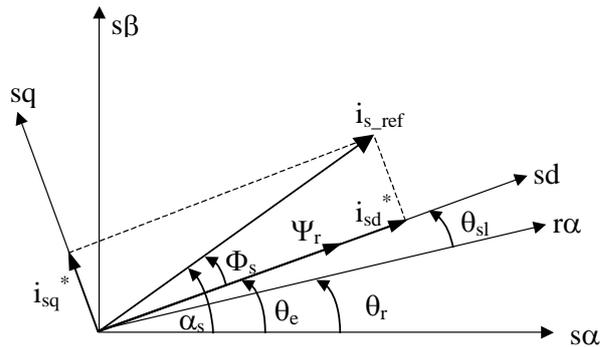
Fig. 5. Position of stator current and rotor flux vectors
