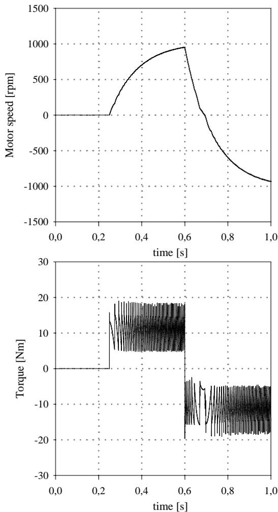
Fig. 6. Motor speed and torque response in open-loop speed control
