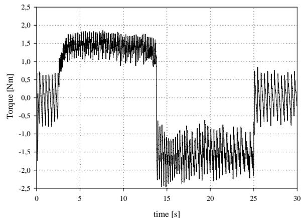
Fig. 2. Torque response in basic DTC drive
