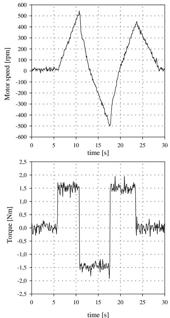
Fig. 7. Motor speed and torque response under square torque command
