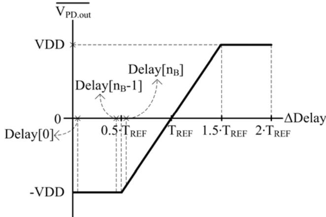
Fig. 5 Output Characteristic of the proposed DET-PD
