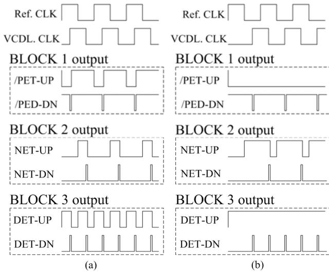
Fig. 2 Timing Diagram (a)  $-\pi \sim \pi$  range (b)  $-2\pi \sim -\pi$  and  $\pi \sim 2\pi$  range
