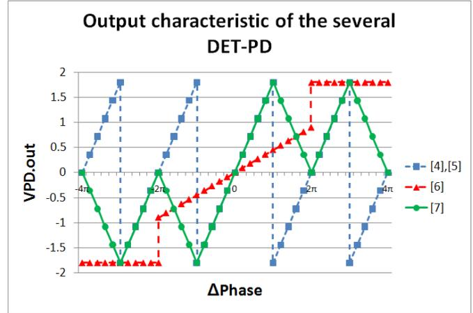
Fig. 3 Output Characteristics of the several DET-PDs
