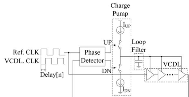
Fig. 4 Block Diagram of Analog DLL
