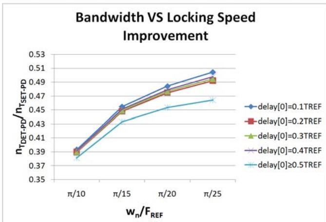
Fig. 6 Locking time improvement according to  $\text{delay}[0]$  and DLL bandwidth
