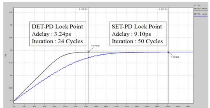
Fig. 7 Comparison of DLL locking process between DLL with DET-PD and DLL with SET-PD
