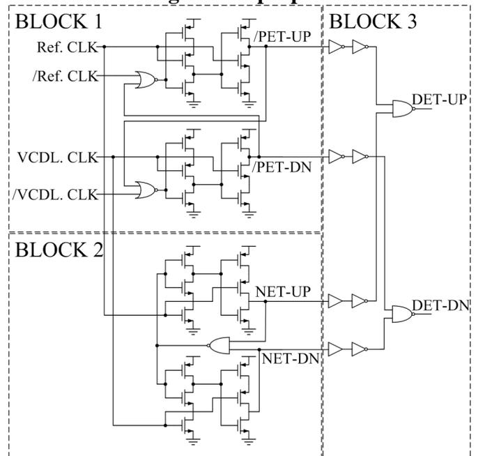
Fig. 1 Overall structure of the proposed DET-PD
