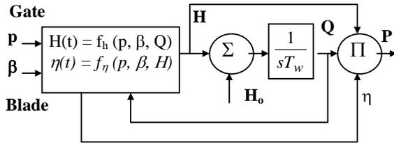
Fig. 2 Conceptual model of a Kaplan turbine
