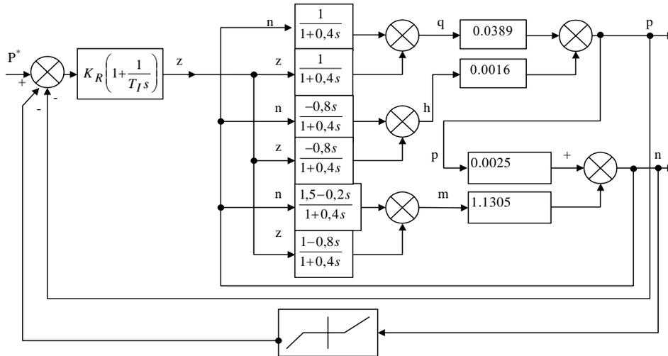
Figure 3. Block Diagram of the control system for hydraulic turbines
