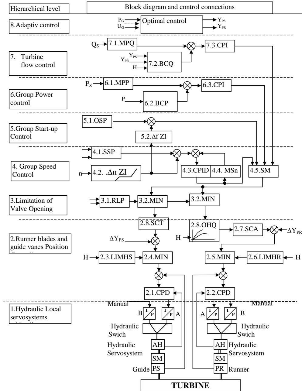
Fig.1. Block diagram of hydraulic turbine control system
