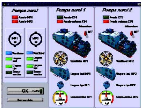
Fig.13. Mud pumps status window.
