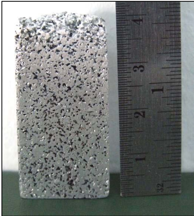
Figure 6 Aluminium foam from aluminium powder 50 mesh
