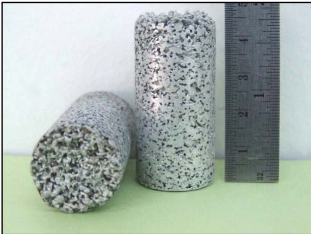
Figure 4 Specimens were cleaned by using a hot water
