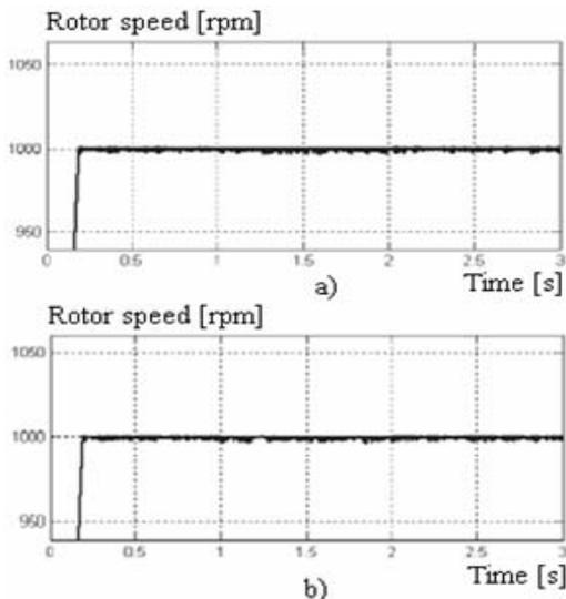
**Fig. 6.** Dynamic performance comparison (Rotor speed) between the classical PI controller (a) and the neural controller (b).
