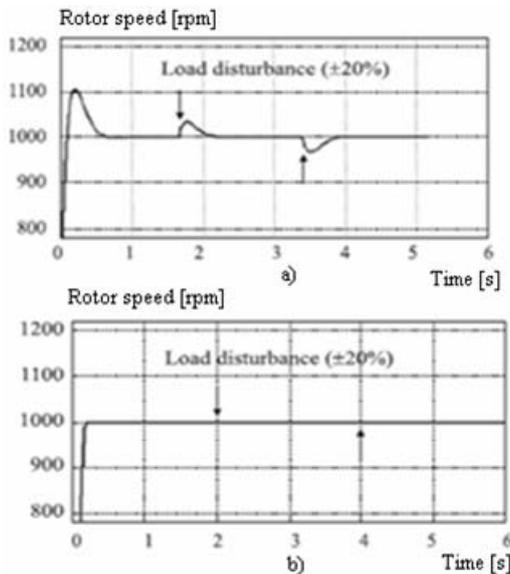
Fig. 3. Comparison performance (rotor speed) between the classical PI controller (a) and the hysteresis controller (b).
