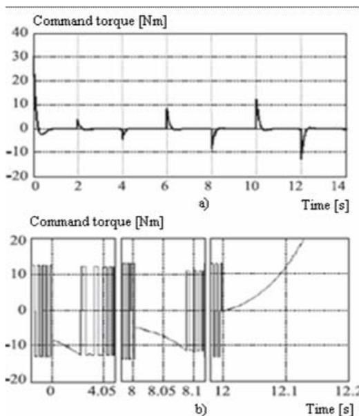
Fig. 4. Comparison performance (command torque) between the classical PI controller (a) and the hysteresis controller (b).
