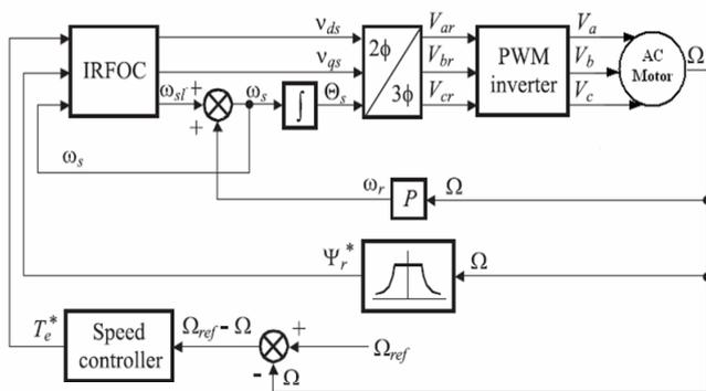
Fig. 1. The indirect rotor field orientation control.
