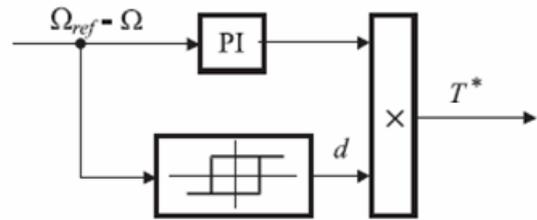
Fig. 2. The Hysteresis PI controller structure.
