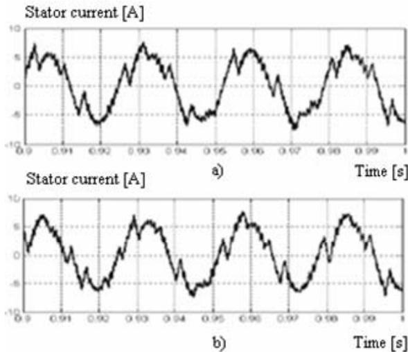
**Fig. 5.** Dynamic performance comparison (Stator current) between the classical PI controller (a) and the neural controller (b).
