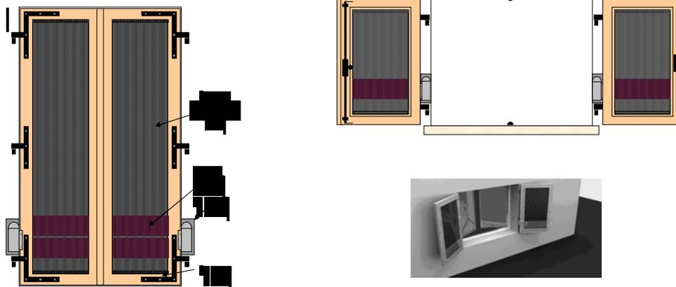
*Figure 3: The new solar air collector: the solar shutter*
