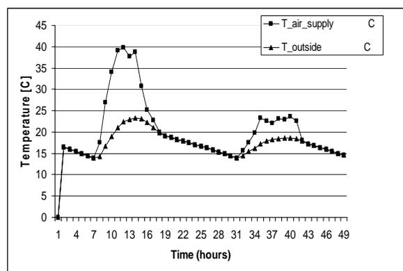
Figure 7: Variation of outside and supply temperatures with solar shutters during a 2-day winter period
