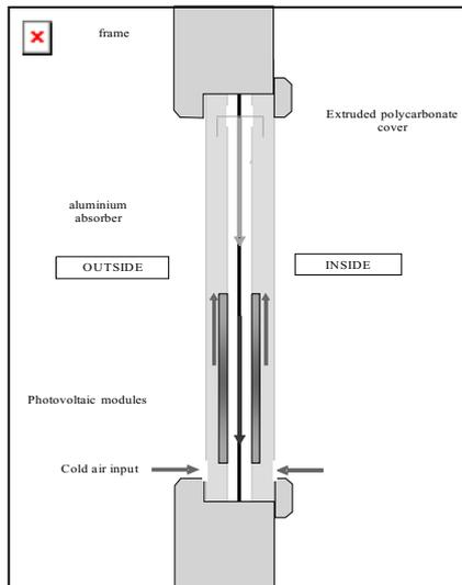
**Fig. 4.** Principle of the new solar air shutter and the air collector: the rotating part on the shutter, the fixed part in the wall and a view of inside house
