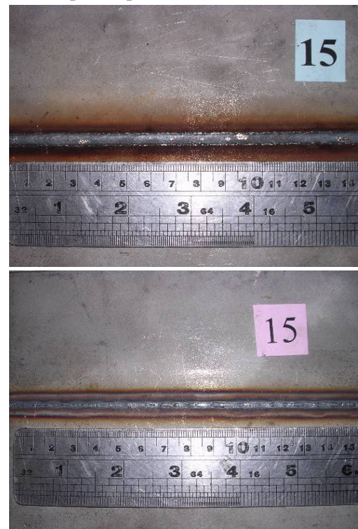
Figure 5 The specimen on higher Ultimate tensile strength by welding parameter on welding current of 90Amp 500 2 welding speed of mm/min shielding gas of Ar+5%O 2 .
