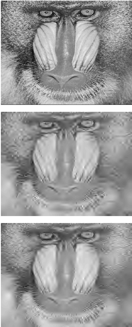
Fig. 2. Coding results of Mandrill image at 0.06 bpp: original (top), SPIHT(middle), Proposed algorithm (bottom).
