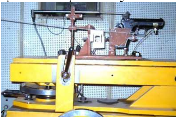
Fig.5 Experimental device for handgun tests
