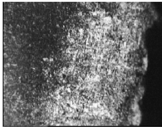
Fig. 15 Sample D–S1; M+D+ T.I.A. (x 200) (decarburated area edge + T.I.A.)
