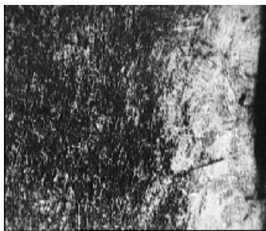
Fig. 14 Sample C – S2; M+D (x 100). (decarburated edge)
