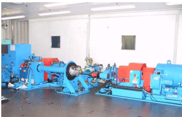
Fig. 1. Virtual engine simulator
