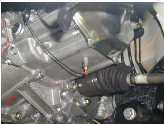
Fig. 4. Acceleration measure point
