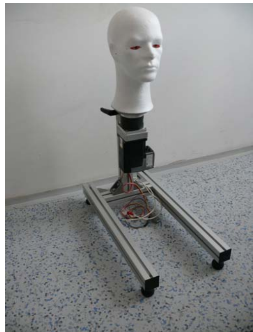
Fig. 10: Model of the head and stepper motor including planet gearbox (verification of rotation measurement)
