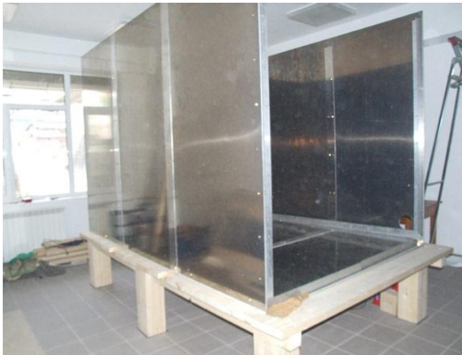
Fig. 5. Shielded room against the spurious microwave signals for radiometric operations
