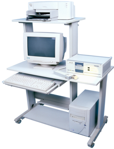
Fig. 7. Installation containing the radiometer and the computer for microwave energy map registering
