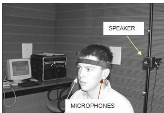
Fig. 2: Empirical HRIR measurement at FIU.
