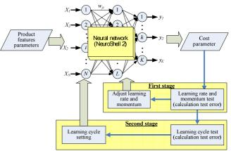
Fig. 9 ANN testing network structure
