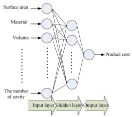
Fig. 5 BPN structure for estimating the cost of plastic injection molded products
