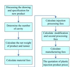
Fig. 3 Cost evaluation procedure for traditional plastic injection industry
