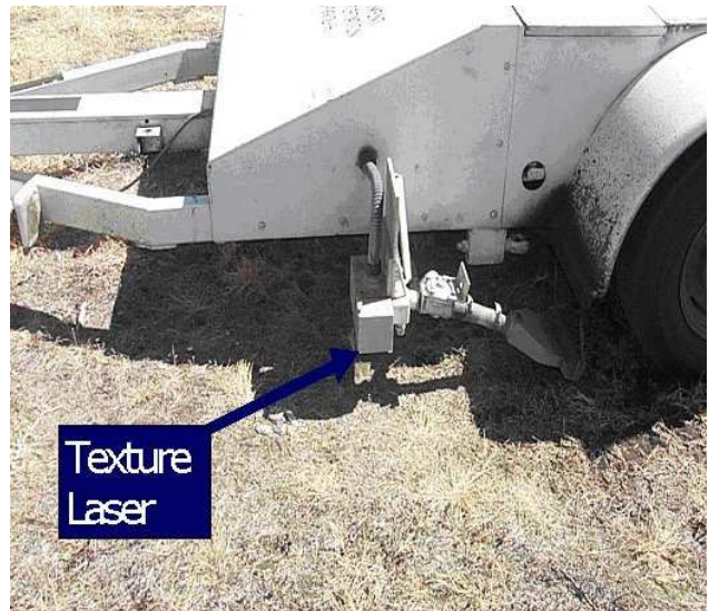
Figure 3 Installation of the texture laser on test trailer during data acquisition.
